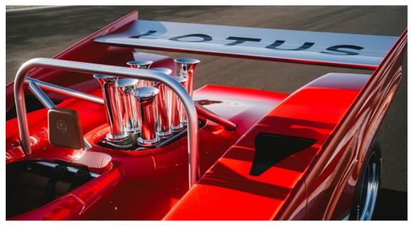
Also improved is the car's mid-mounted, period-representative V8 push-rod engine, which aims to put out more than 830bhp at 8,800rpm. The iconic Can-Am-inspired air intake trumpets are obviously the Type 66's party piece, which not only look amazing, but help improve the power output too. Overall, the Type 66 is a truly stunning work of engineering, and a car that would have surely struck fear in the hearts of its Can-Am competition.
